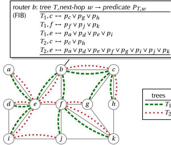
Figure 3: Multi-Tree Routing Scheme
