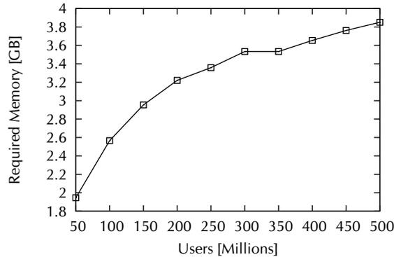
**Figure 12:** Scalability of the Memory Requirements (One Tree on AS 3257)
